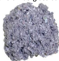
Cellulose is often sprayed over old fiberglass batts
